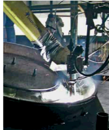
Rebuilding a grinding table with KALMETALL W100.
