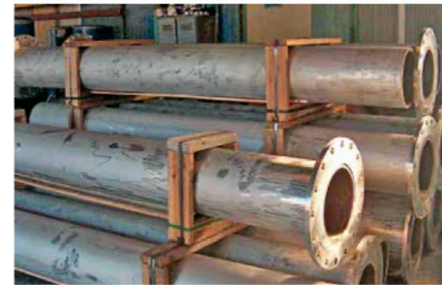
Down pipes of a direct reduction line made of KALMETALL W151, 355 mm diameter; basic material 1.4829 of 12.8 mm
