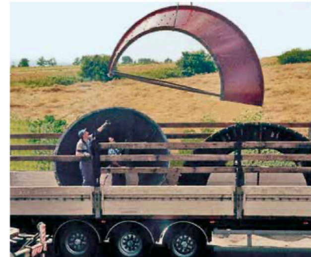
Cyclone separator cones of KALMETALL W100 6 + 4 fixed by means of bolt welding
