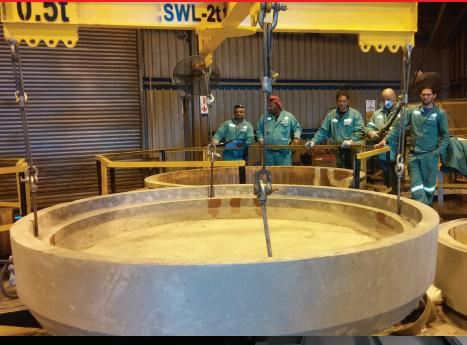
The company's precast facility is adequately equipped with overhead cranes, that are capable of moving and hoisting big blocks from the casting area, to the drying furnace or load finished products onto trucks.
