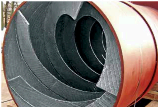
Feed screw for mill inlet cylinder, protected with KALMETALL W100, diameter 1,350 mm, lining thickness 5 or 8 mm, self-supporting construction
