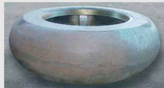
Kalenborn supplies grinding rolls, grinding tables and mill linings for grinding plant used for raw material, coal and clinker. Top: regeneration of a grinding roll with KALMETALL W100, bottom: newly cast component made of KALCAST C153 hard casting, each 1,500 mm Ø.
