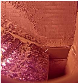
The Endoscopy offers high-quality images thanks to Full HD video cameras integrated into the cooling jacket. The furnace can only be observed using the digital video module, which allows all images to be viewed simultaneously on a computer or tablet. With its water and air-cooled housing, the Endoscopy can operate in furnaces with temperatures up to 1600°C.
