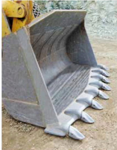
Loading shovels are subject to increased wear in quarries. Therefore, linings made of KALMETALL HB, KALMETALL and KALCAST provide good protection.
