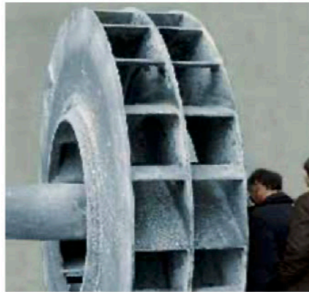
Fan housings and rotors to be integrated in pneumatic systems are reliably lined with KALMETALL.
