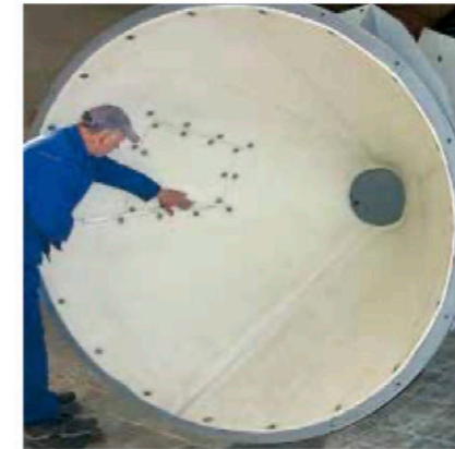
Slide promotion lining of a silo outlet with KALEN 1000 slide promotion plastics.
