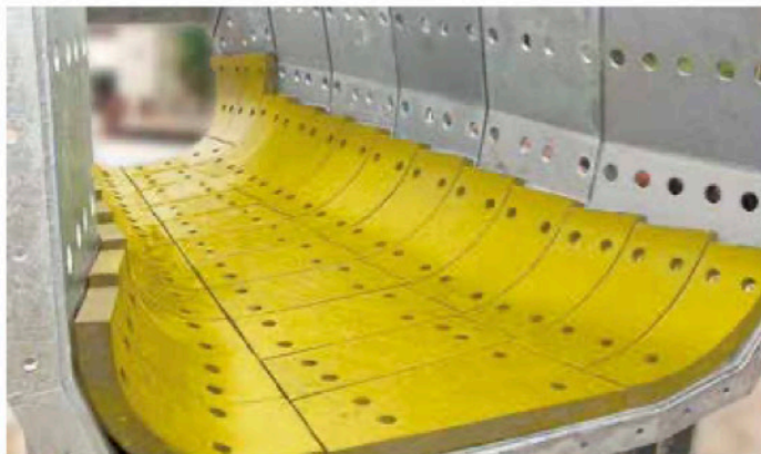
Reliable protection in a material chute with 62 mm thick KALCAST 155 castings. For improved impact resistance and noise level, an 8 mm thick rubber layer is installed beneath the castings.
