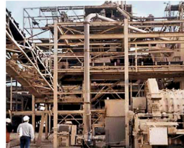
The best possible protection for hydraulic pipes used in the classification of ores is ceramic materials. This can be ABRESIST, KALCOR or KALOCER.
