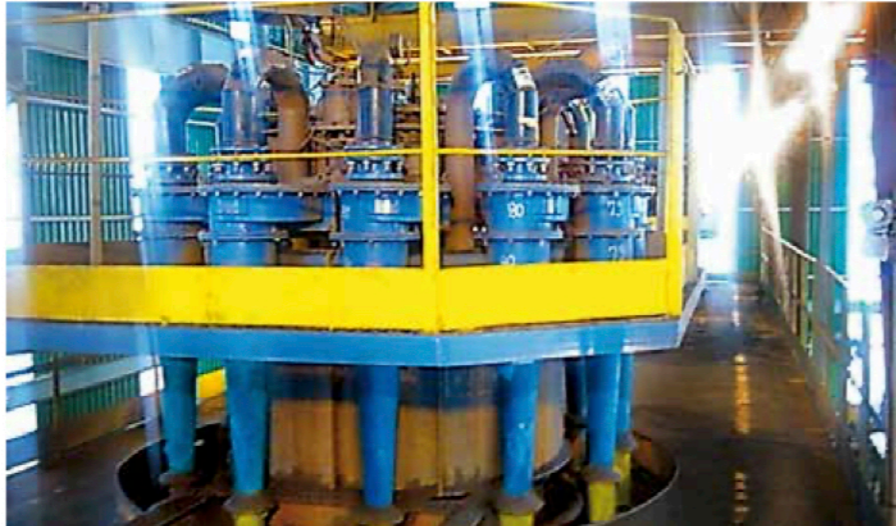
Proper wear protection of hydrocyclones extends the service life of the equipment and reduces the cost of downtime
