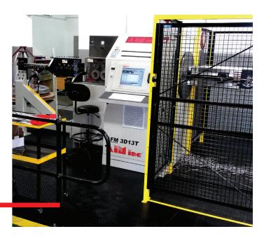
Dickinson Industries (Pty) Ltd uses wire coils that adhere to strict internal material specifications and has undergone the annealing process. Anchors are produced by means of free bending on a CNC-3D bending machine, thereby ensuring that the anchors meet the required high quality standards.
