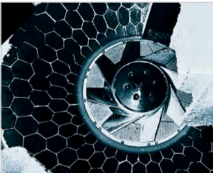
Waste paper bales are mixed for paper recycling in pulpers. Since the bales contain considerable impurities the pulper bottom is durably protected with ABRESIST.
