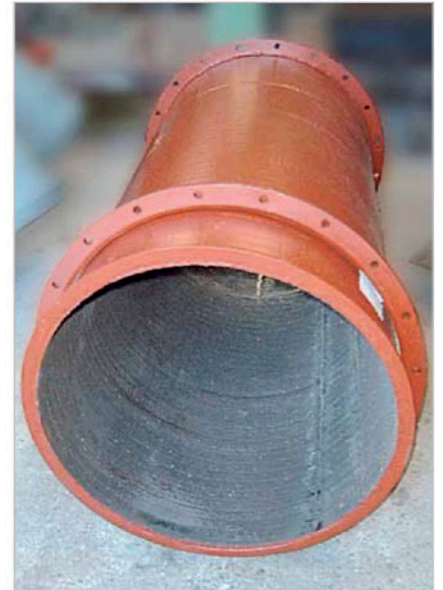
Pipe armored with KALMETALL-W 100 installed in a dust collecting system; inside diameter 400 mm, system thickness 8 + 5 mm
