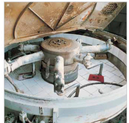
Agitators and mixers subject to extreme wear can be durably protected with KALOCER tiles shaped to the specific equipment design
