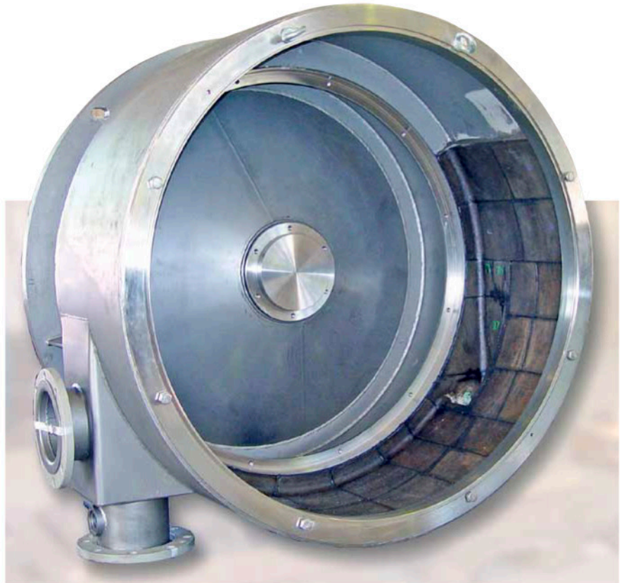
Combi-sorter made of high-grade steel used by the paper industry – protected from wear by fused cast basalt tiles
