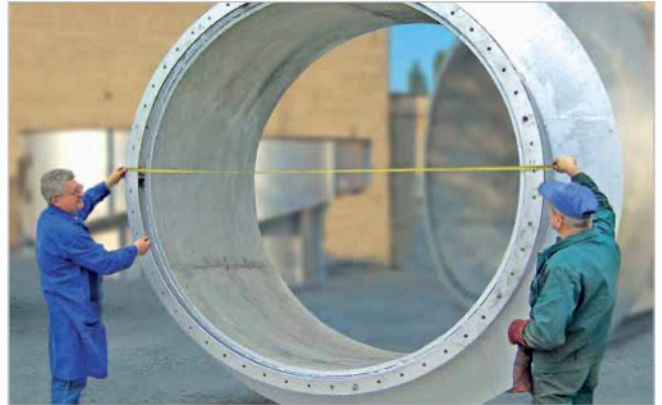
Separator of a cement mill lined with KALCRET-BNX, up to 3,200 mm diameter
