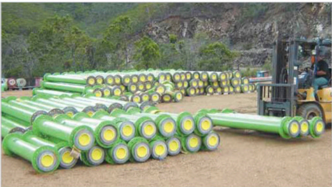
Highly abrasion resistant KALOCER pipes to transport ore sludge in a mine in the Far East
