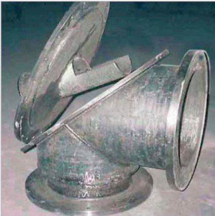
Pulverized coal burner lined with KALMETALL-W 145
